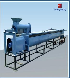
Additionally, this machine also has the advantages of low off-gas emission and complete removal of the exhaust gas. It is a kind of chemical equipment with high efficiency, low energy consumption and compact structure. Maintenance of the equipment is easy. Paddle Dryer are used for a wide range of application e.g. Agricultural, chemicals, petrochemical, detergents, food products, herbs, s, minerals, metal, pharmaceuticals, Polymers, etc.
